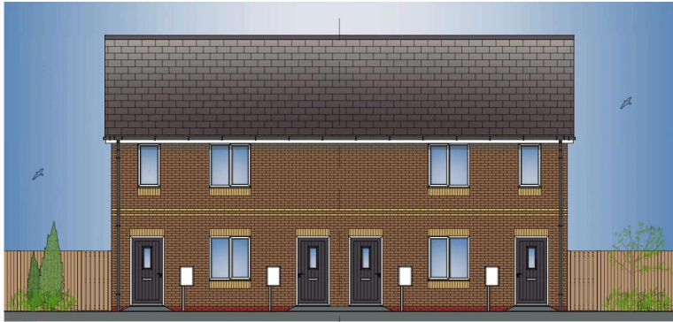
Type P1 & P2 Front Elevation - 1B2P Maisonette 50 & 57 1 Bedroom 2 Person Maisonette (50m 2 & 57m 2 )
