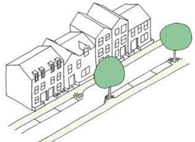
Figure 21: Integrated traffic calming measures such as street trees and chicane in the road
