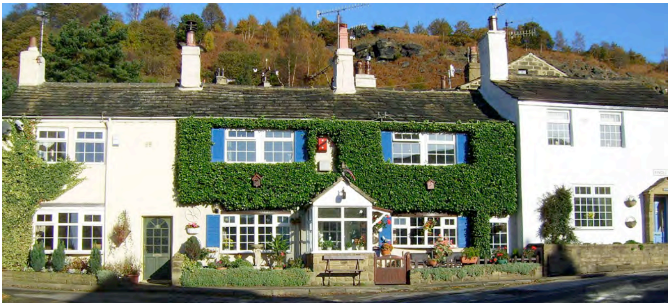
4-6 Knoll View retain important features such as stone slate roofs, corniced chimneys and most of the original fenestration, but alterations such as the rendering of the stonework and modern doors and windows have undermined their traditional character.
