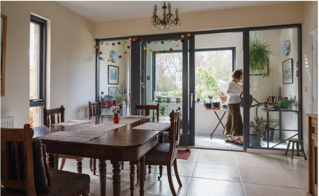
The Derwenthorpe development includes many innovative examples of energy efficient design. The homes have a highly efficient building fabric and are carefully orientated to ensure large windows face south to maximise solar gain. Many houses include sunspaces, offering a buffer between inside and out, collecting solar energy in the winter and cooling homes in the summer. Heating and hot water is provided from a biomass-fired district heating network which forms part of the development.
