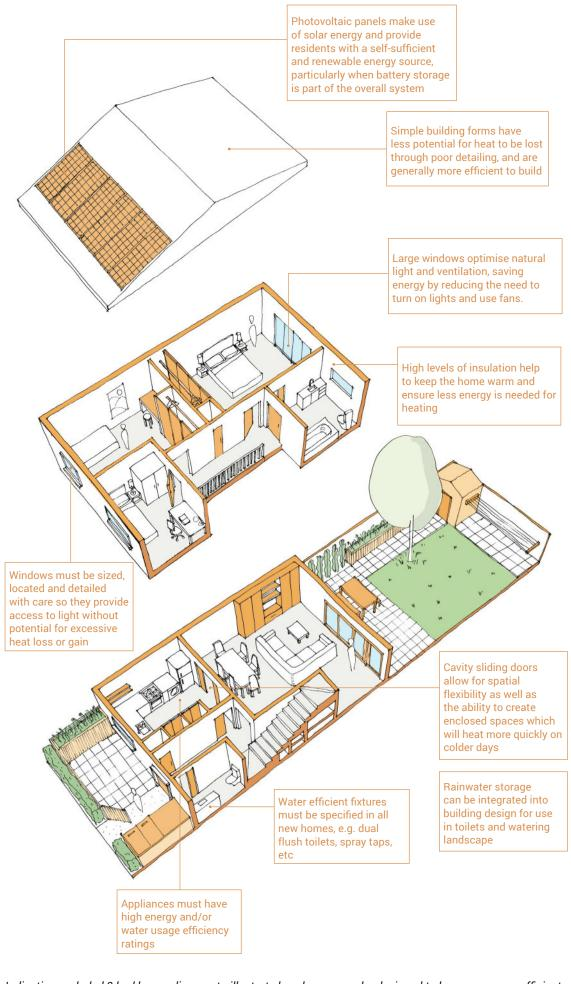
Indicative exploded 3 bed house diagram to illustrate how homes can be designed to be more energy efficient
