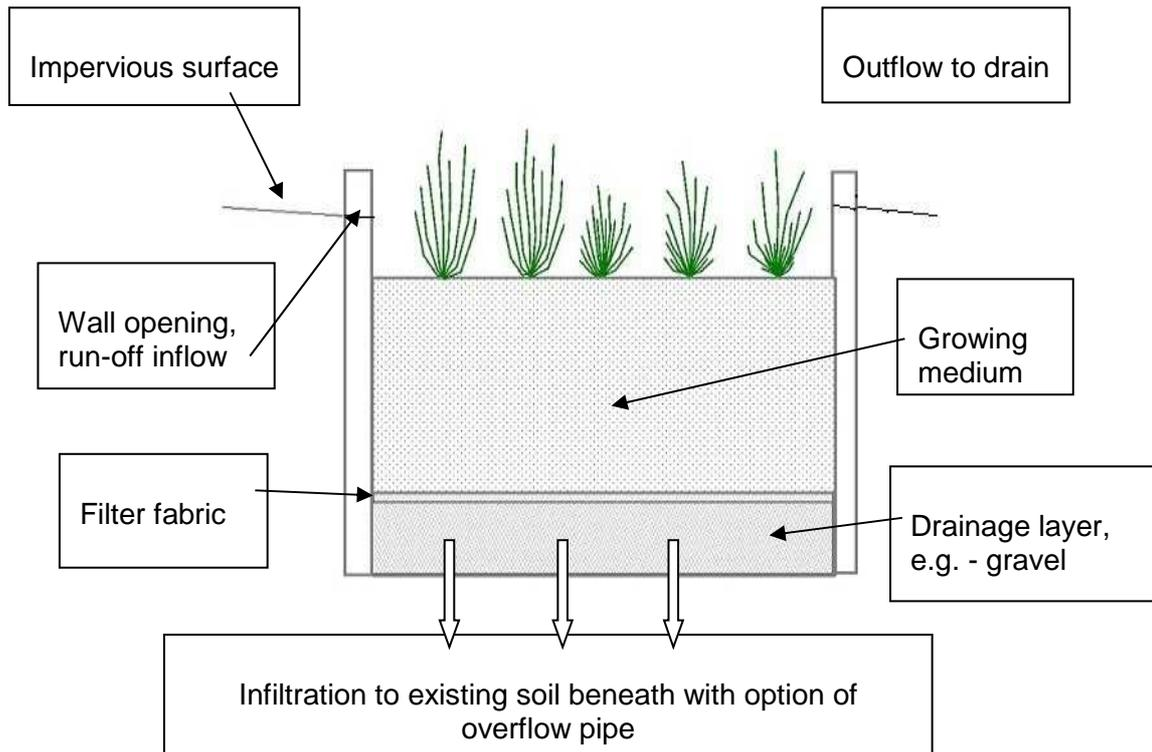
Figure 67 –side profile of an infiltration stormwater planter.
