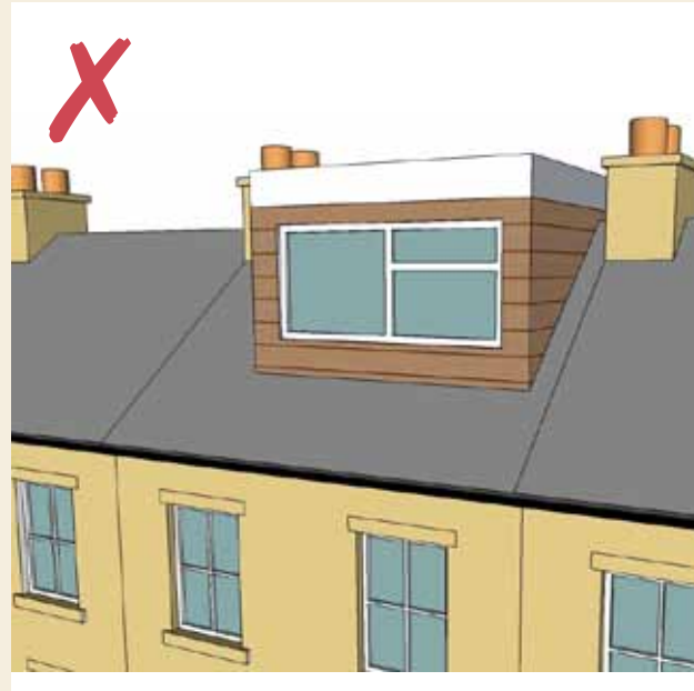
Figure 45: Unacceptable – above ridge, too large, poor materials, poor window details
