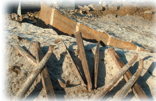
Tools of the trade. Plugs and feathers rest on rock which has been recently split
